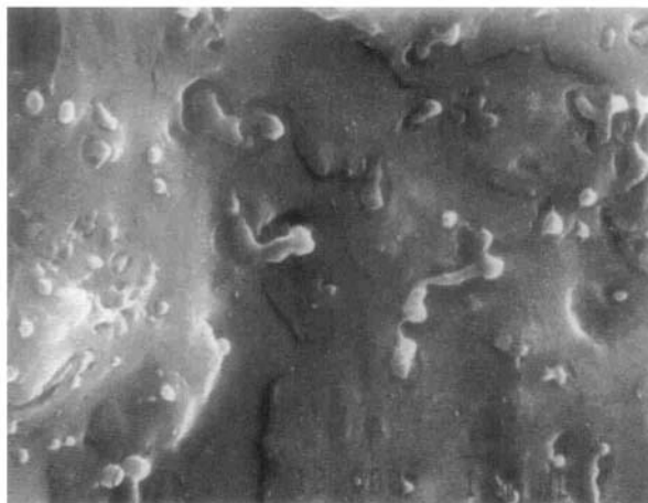
Figure 6 Scanning electron microscopy (SEM) micrograph of the LDPE/PP 25/75 blends modified by 1 wt % peroxide ( \times 10,000 ).
