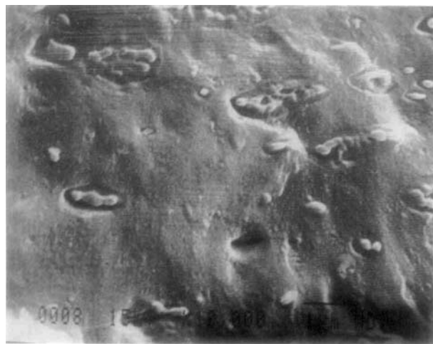
Figure 5 Scanning electron microscopy (SEM) micrograph of the LDPE/PP 25/75 blends modified by 30 kGy irradiation ( \times 10,000 ).
