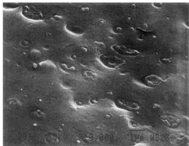
Figure 3 Scanning electron microscopy (SEM) microphotograph of the LDPE/PP 25/75 blends prior to modification ( \times 10,000 ).
